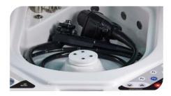
The endoCleaner is optionally equipped with a signal system to monitor the flow through each channel of the endoscope, ensuring quality cleaning and disinfection during the treatment cycle.
